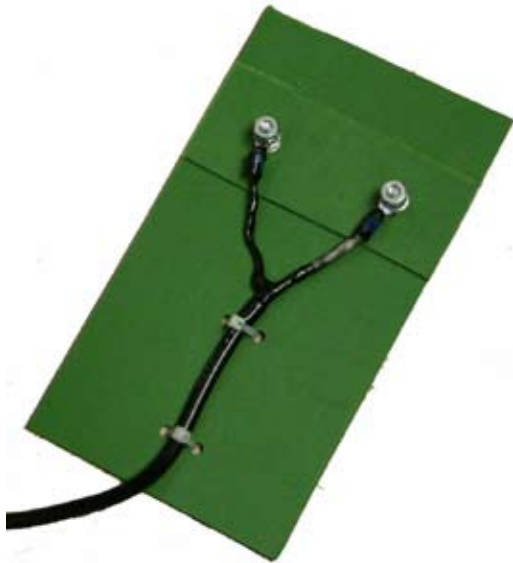
Figure 4 - Coaxial cable center conductor and braid treated with Liquid Tape and mounted to a piece of plastic using ty-wraps for strain relief.
