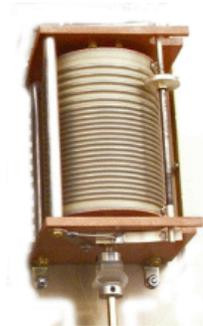
For capacitor value, look for something with a top range of 200 – 500 picofarad (pf) and for an inductor - 28 – 55 microHenrys (uH). If most of your operating is done on the lower bands go for the larger sizes. On the other hand, if your preferences are for ten meters, build with the smaller.
