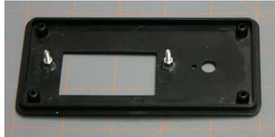
Photo 3 – Inside cover showing studs for meter mounting.
