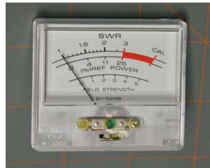
Photo 4 – Old meter as it came from the SWR meter.
