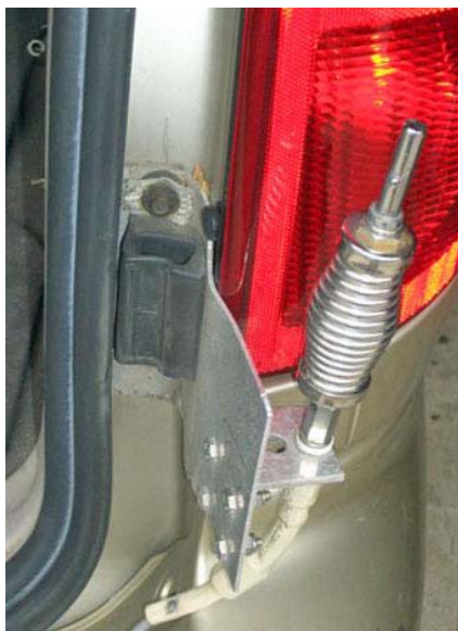
Antenna connection on N3HS's van
