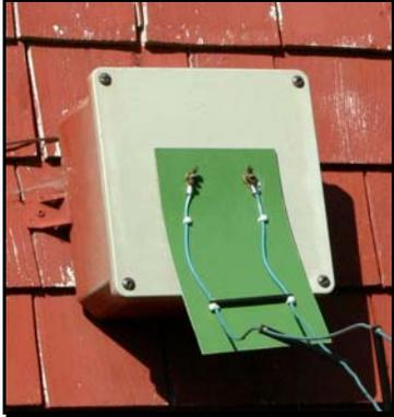
Figure 10 – Strain relief on the transmitter end. Inside the PVC box are threaded 1/4" steel rods in PVC pipe going through the wall to the tuner.
