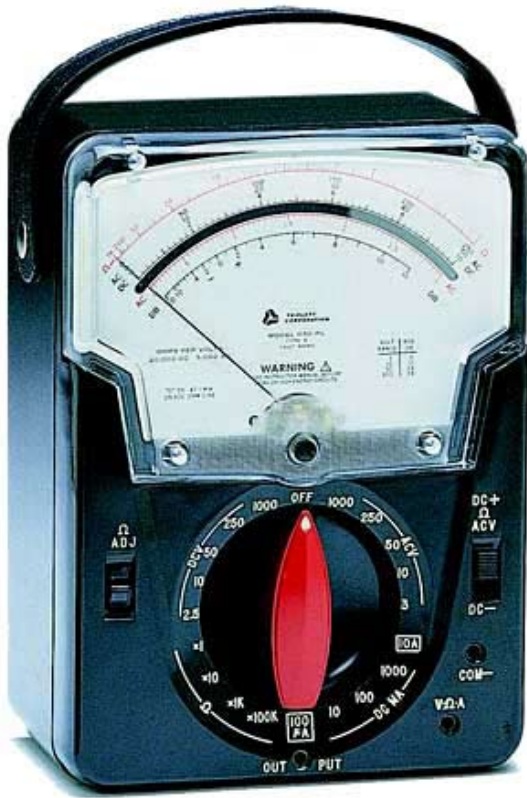
Figure 1 - Triplet 630 meter. Note the mirror in the middle of the scales. This allows the user to read the measurement more accurately. The pointer and the mirror image are aligned so that the image is hidden by the pointer. The correct measurement is then read from the appropriate scale.
