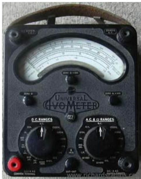
Figure 4 - The British manufactured AVO Model 8 MkII meter (commonly called the 'AVO'). The name stands for Amps/Volts/Ohms. In 1970, a new Model 8-Mk4 sold for about $175. Today the current version goes for about $875. Better look on E-Bay! I used one of these in my first job in the late 1960's fixing car and two-way radios.
