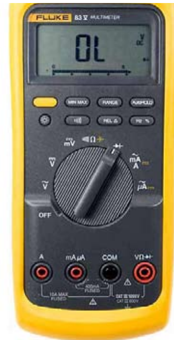
Figure 2 - Fluke 83V digital meter. The accuracy when measuring volts DC is +/- 0.01%. The unit is auto-ranging. Simply set the switch to whatever you want to measure, apply the test leads, and the measurement appears. No switching to get the reading in the high end of the scale as you would with an analog meter.
