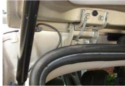
Figure 8 – View of grounding strap on the rear hatch hinge and the coax to the VHF/UHF antenna.
