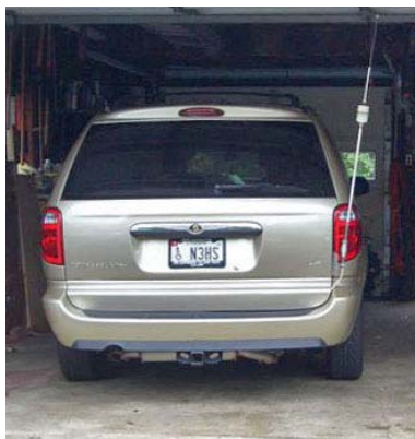
Figure 11 – Rear view of the van showing the Hustler HF antenna.
