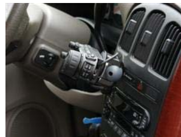
Figure 5 – Side view of the control head mounting arrangement looking toward the steering wheel.
