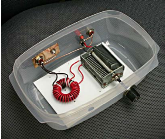
Figure 13 – High impedance output tuner built from the circuit in figure 11 and housed in a Rubber Maid food storage container. The copper wire under the two sets of connectors was a common ground for experimenting and has since been removed.
