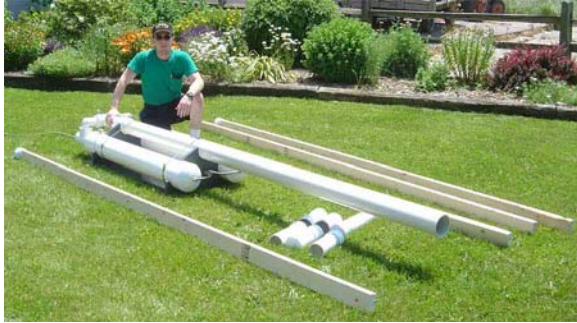
Figure 3 – The caption from the spudtech.com website reads, “Above is a picture of the massive custom air cannon that was built for the US Dept. of Agriculture a few years back. It’s a tornado simulator designed to fire a 12 foot long, 15 pound 2 x 4 at a wall at 100 MPH.”
