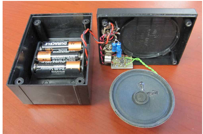
The LM4861 tracer shown with the case open. Three AA batteries in the bottom part provide the power (4.5 VDC). They are connected to the off/on switch on the rear of the volume control. Signal is input via the 1/4 inch jack through the parallel capacitors, to the volume control, and finally to the circuit board shown above the speaker. A square of soft foam (not shown) fitted on top of the batteries holds the speaker in place in the case front once the halves are assembled.
