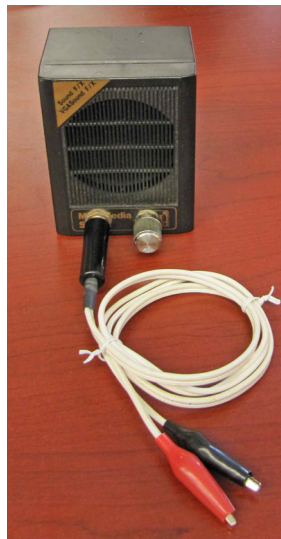
The LM4861 signal tracer built into an old computer speaker housing.
