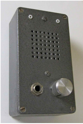
The LM386 signal tracer in a Hammond aluminum box. The two white connectors at the top are wired to the speaker terminals. See the June issue of the newsletter for more information on this model.
