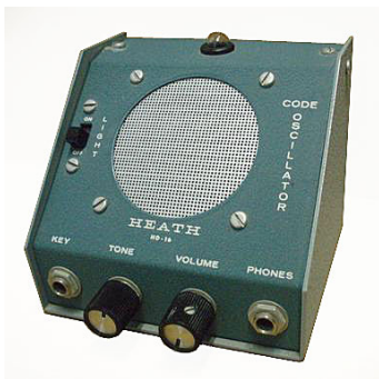
Grandma's old Heath HD-16 code practice oscillator
