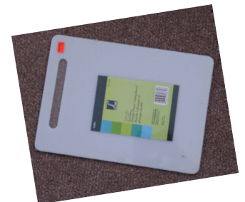
Use a cheap ($2) plastic cutting board for insulator material
