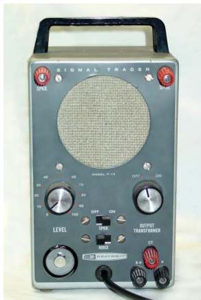
The Heathkit IT-12 Signal Tracer. Note the 'magic eye' tube in the lower left corner.
