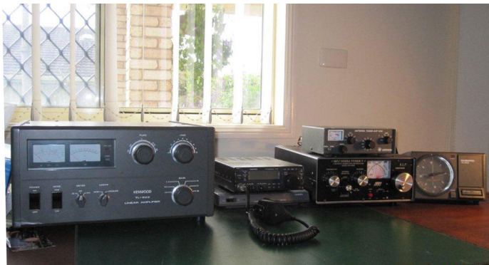
VK4XH's present HF station from L to R - TL922 1200 watt Power amp, TS 50 Tcvt, switching power supply for TS 50, 200 watt and 3 KWatt tuners, and the rotor for the beam. Not in Pic but inside his car is an 857D Heathkit TCVR with an Atas 120 auto tune antenna. He also has IRLP capability on Node number 6139 with which he uses a VX5 Yaesu handheld.
