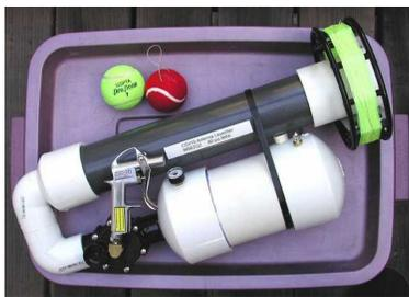
A tennis ball launcher from www.antennalaunchers.com with a bow fishing reel on the end of the barrel.
