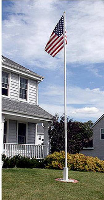
A flagpole installation at KX9DK using a Hustler 4BTV trapped vertical antenna inside plastic pipe. As with N4AQ's antenna, he omitted the antenna's capacitance hat.
