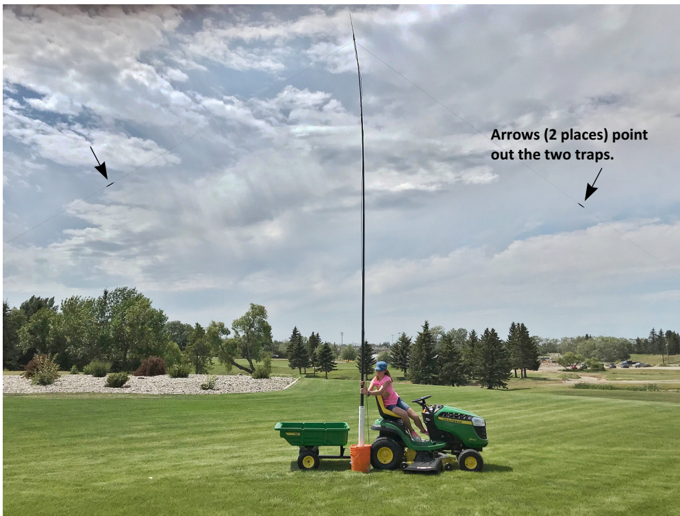
Figure 3 - Bucket, holder and mast supporting trap inverted-V antenna. I tried it with just the bucket but there was a breeze blowing and it kept tipping over. I enlisted the lawn tractor as a support but the wind defeated that. My grand daughter volunteered to provide additional support for the test. In return, she got to drive the John Deere around the lawn.
