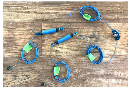
Figure 1 - Trap 40/20 antenna assembled but not trimmed to resonance. Shrink tubing has not been placed over traps.
