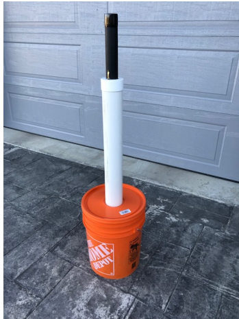
Figure 2 - Weighted bucket with pipe and cap originally used to support the squid pole vertical antenna is being re-purposed for the center support of the trap 40/20 meter dipole/inverted-V.
