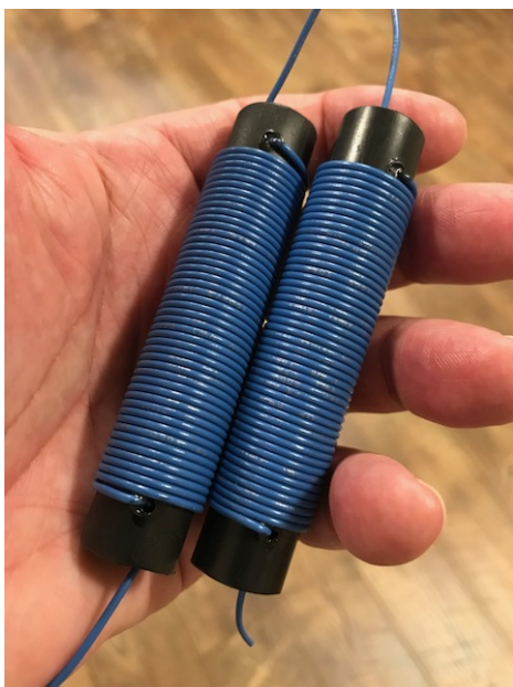
Trap coils after winding. Liquid Electrical Tape has been applied to the wire where it passes through the holes. The wire has not been trimmed to length to fit into the printed circuit boards.
