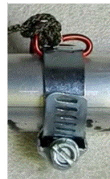
Figure 3 - Two views of the guy line tie point made from copper wire and a hose clamp. Three of the formed wire pieces would be equally spaced around the clamp.
