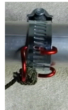
Figure 3 - Two views of the guy line tie point made from copper wire and a hose clamp. Three of the formed wire pieces would be equally spaced around the clamp.
