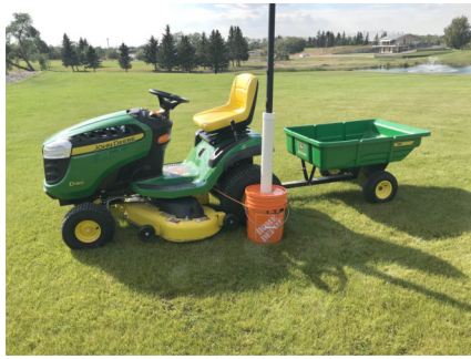
Figure 3 - Bucket with pole strapped to the side of the lawn tractor wheel with bungee cords.
